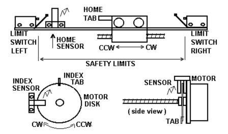
ABORT LOOP FUNCTION. In TMG systems, the ABORT loop is used to remove all winding power to the motor during an out-of-bounds condition. The ABORT feature can be used to provide hard-limits, emergency stop, door inter-locks, and other safety features. As the ABR input, to the driver, must be LO (ground) for the driver to step; opening the loop will stop (free) the motor regardless of the control logic. The diagram is typical of TMG "Fail-Safe, Hard-Soft" limit loops.
